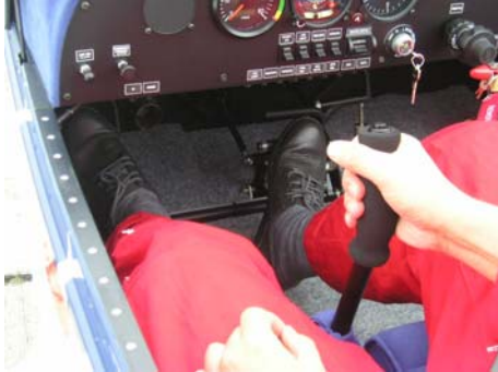
Picture: Left rudder pedal deflected forward– airplane yaws and banks left
