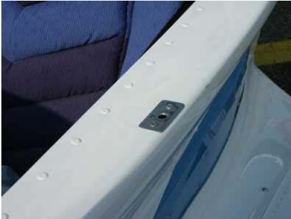
Picture: Holes to fit the side center pins of big-bubble canopy
