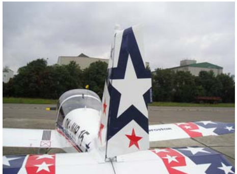
And corresponding deflection of rudder to the right.
