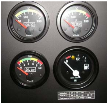
Picture: Detail view of engine analogue instruments-color markings
