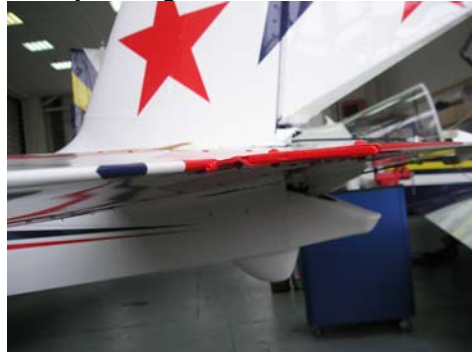
Picture: Trim tab deflected in Nose heavy position
