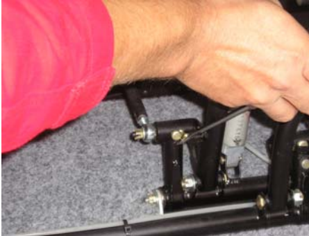
Picture: 1 Push the locking pin sideways.
