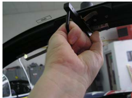
Picture 4: Closing the canopy from within
