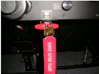
Picture: Ballistic system ejection lever
