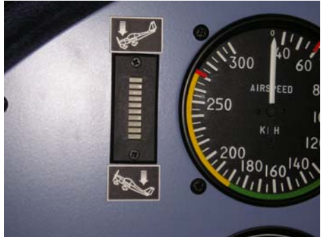
Picture: Trim tab position indicator on instrument panel
