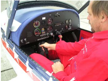
Picture: Longitudinal control (control stick) forward- airplane descends
