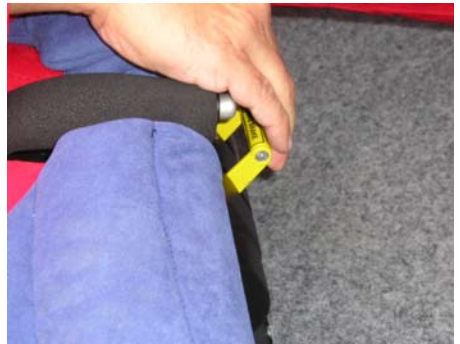
Picture: Parking brake ON
