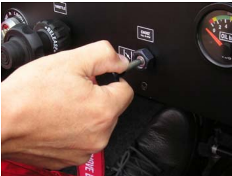
Picture: Choke control lever (push-pull type)
