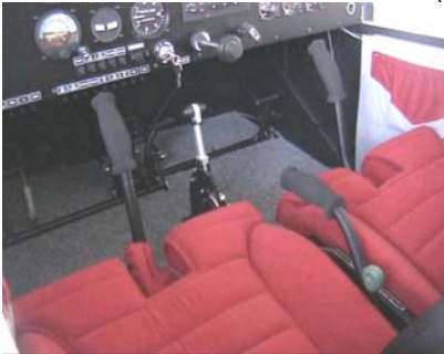
Picture: Wing flap control lever located between the seats
