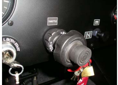
Picture: : Throttle lever set for max. power
