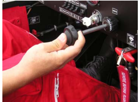
Picture: Rough setting of engine power
