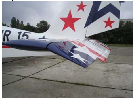
Elevator deflection with control stick fully forward
