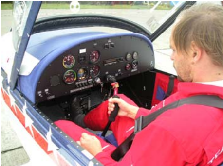
Picture: Stick deflected right – airplane banks and turns right
