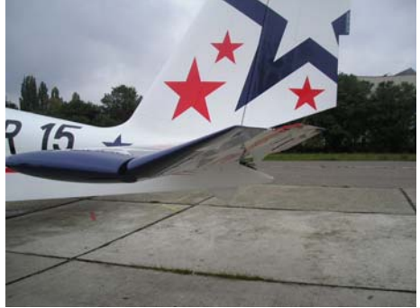
Elevator deflection with control stick fully aft
