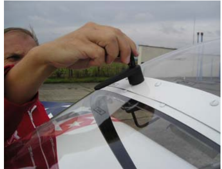
Picture: 2 Use the key to unlock the canopy lock
