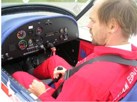
Picture: Longitudinal control (control stick) aft- airplane climbs
