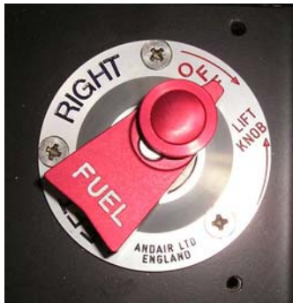
Picture: Fuel selector in closed position
