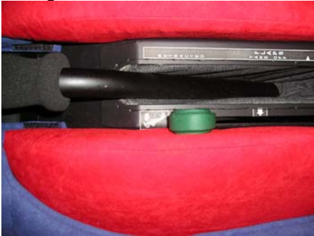
Picture: Green elevator trim tab control lever set to Nose heavy position
