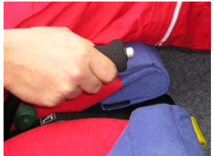
Picture: Set the lever to desired position. The lever should be automatically locked in that position
