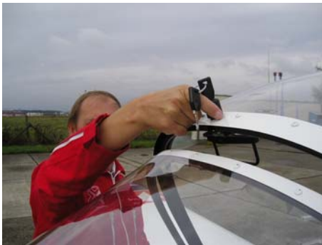
Picture: 3 Turn the lock lever and slightly open the canopy
