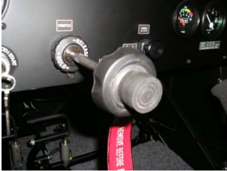
Picture: Throttle lever set for idle
