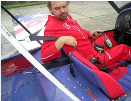
Picture: Headset jacks connected to the sockets behind the right seat back. The two left are for co-pilot headset
