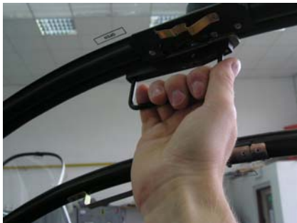
Picture 1: Closing the canopy from within
