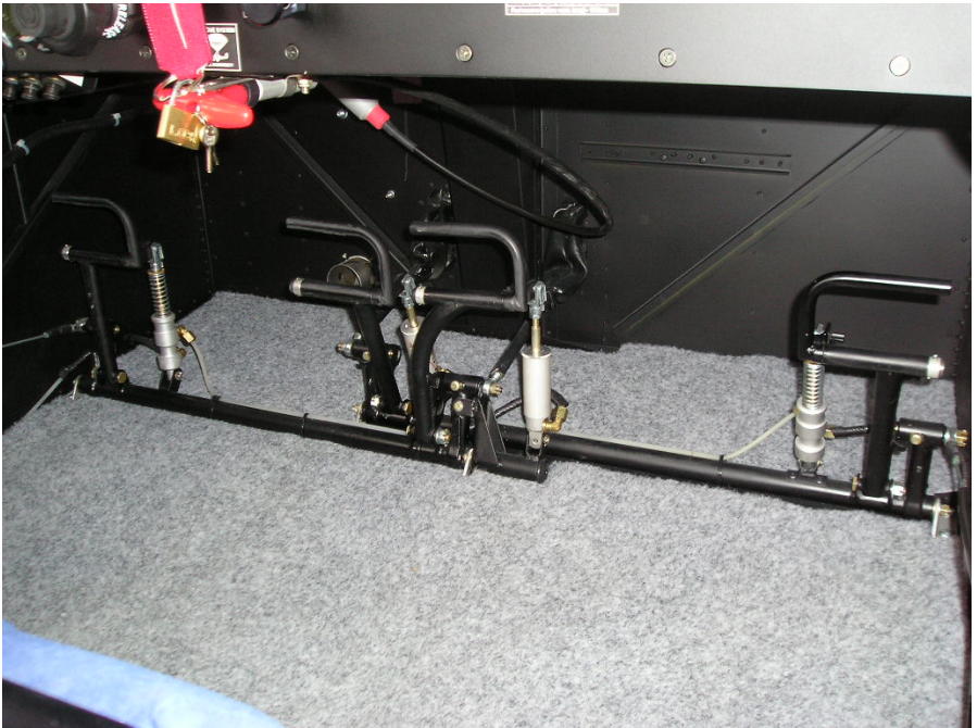
Picture: Dual rudder pedals with toe-brake pedals on the top.
