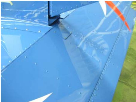
Picture: Elevator upper skin with a square cover of trim servo
