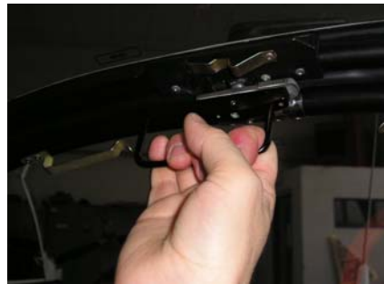
Picture 2: Closing the canopy from within
