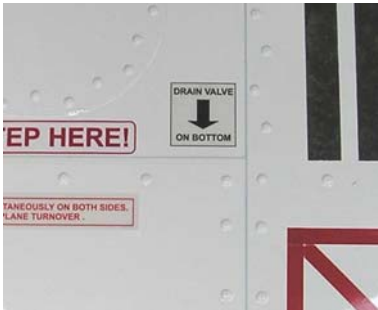
Picture: Placard-arrow marking location of drain valve
