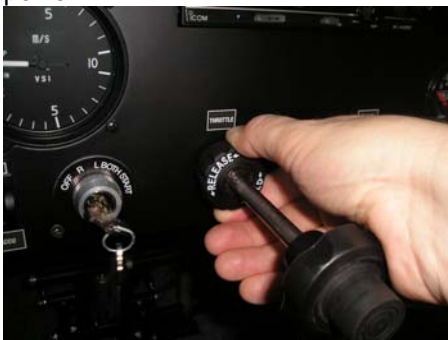
Picture: Friction wheel of throttle lever
