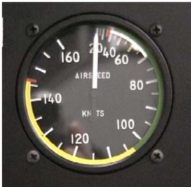
Picture: Airspeed indicator marked with color coded arcs
