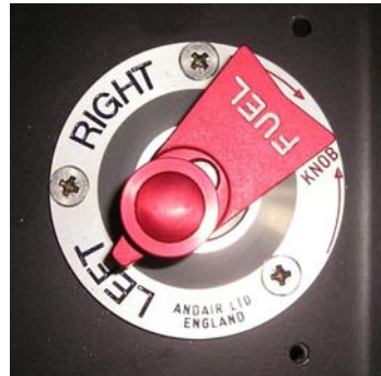
Picture: Fuel selector in left tank position
