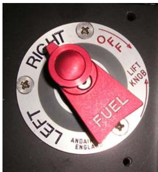
Picture: Fuel selector in right tank position
